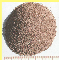
5g of Umoplast: approx 25,000 microgranules 90% between 0.5-1.0mm
